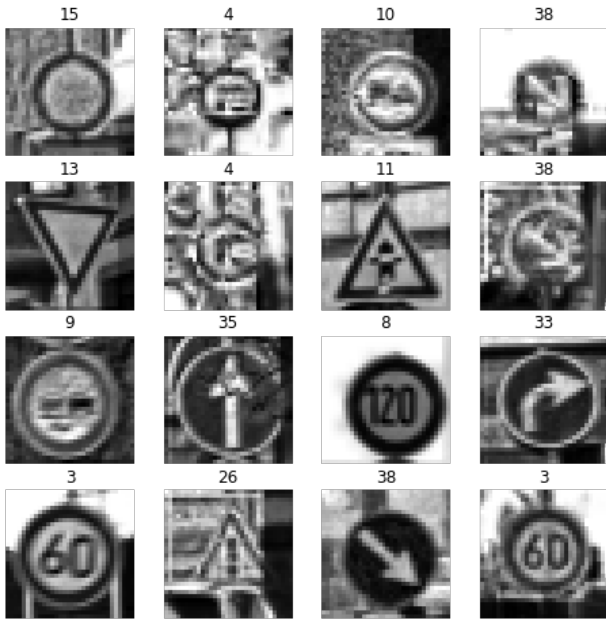
Fig. 18. A subset of images from the Test data-set after applying Contrast Limited Adaptive Histogram Equalization
