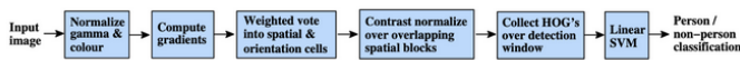
Fig. 11. The original process implemented for human body detected as originally proposed by Dalal and Triggs [4]
