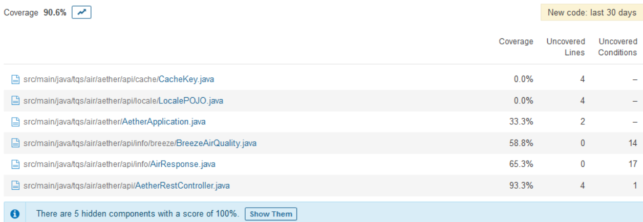
Figure 47. The line coverage per class on our project. The CacheKey and LocalPOJO classes show a 0% coverage, but this is because they possess no methods other than their constructor. We found that it would be redundant to make a test class exclusively for this as these classes are already instantiated in other tests, and if we did write them, we wouldn't be ascertaining nothing new, and would just be doing it to increase the overall coverage metric, hence defeating the purpose for tests. Other than that note how most of our classes possess a coverage of 100%
